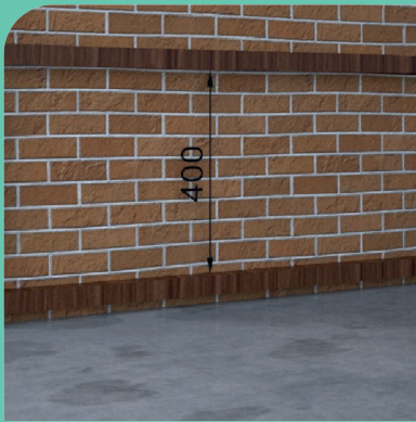
1) Install wooden / aluminium or composite battens to desired area at 400mm centres.
