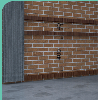
2) Please ensure where boards butt together additional battens are added as per photo.
